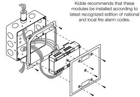
**GSA-MAB:** mount the UIO motherboard inside a suitable Kidde enclosure with screws and washers provided. Plug the module into any available position on the motherboard and secure the module to the motherboard with the captive screws. Wiring connections are made to the terminals on the motherboard (see wiring diagram). UIO motherboard terminals are suited for #12 to #18 AWG (2.5 mm<sup>2</sup> to 0.75 mm<sup>2</sup>) wire size.
